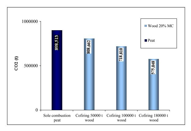
Figure 7.2.3. Potential CO<sub>2</sub> reduction with co-firing peat with recovered wood.
